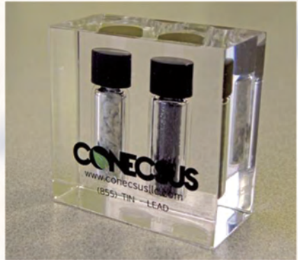
Vial of shredded contaminated trash (left) and the same material now carbonized (right) and converted to a metals-recovering reagent in the RACS process.
